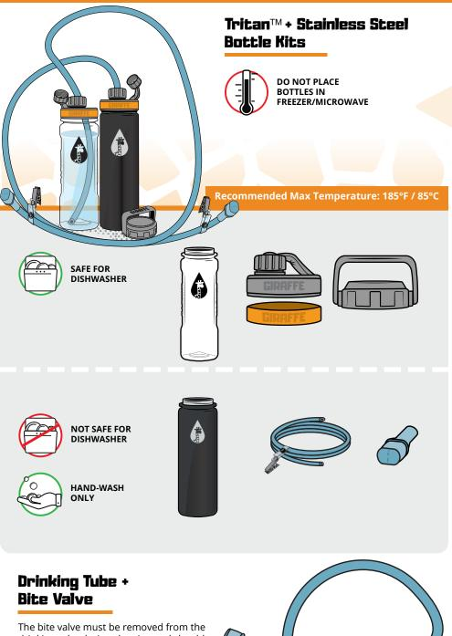
The bite valve must be removed from the drinking tube during cleaning and should **NOT** be pierced with a brush.
